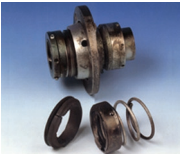
DAMAGED MECHANICAL SEAL
